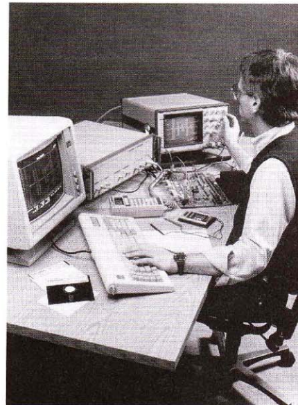
Custom waveforms can be captured by a digital scope or digitizer, and then edited and regenerated with the Series 9100 AFGs. Or, they can be created from scratch from simple elements or equations with our user-friendly EASYWAVE® software.
