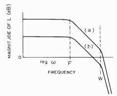
Fig.5. Graphs illustrating that variations in zero-frequency loop gain can cause instability. Curve (a) crosses the 0dB point (unity-loop gain) with a slope of 12dB per octave corresponding to a loop phase shift of 180 degrees. Curve (b) is stable because the loop phase shift is 90 degrees at unity loop gain.
