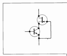
Fig. 3. Bipolar f.e.t. cascode arrangement.
