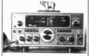
allband, HF, 300 wattstransceiver, 160 / 80 / 40 / 20 / 15 / 11 / 10A / 10B / 10C / 10D / WWV, modes FSK, USB, LSB, CW, AM, with separate 8 pole X-tal lattice filters for each mode fitted. Further features: Side tone at CW, VOX (automatic transmit-receive by talking into microphone), 11 meter CB band, all channels easily selectable through digital counter, excellent receiver sensitivity at extreme crossmodulation security by application for the 7360 low noise beam, deflection mixer tube.
