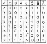
Table 7. Using the complementary outputs of a chain of flip-flops to count down.
