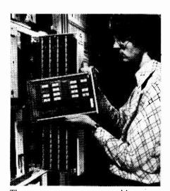
The new m.o.s. reprogrammable read-only memory store for STC's semi-electronic telephone exchange, TXE4A. The threaded wire equivalent used in TXE4 is in the background. As a whole TXE4 saved around 20% of space on Strowger, and the new version saves a further 20% on that. Both memories contain the programme for the exchange's main control unit which establishes the routing of the calls through the exchange.
