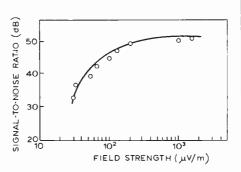
Fig. 3. Receiver signal-to-noise output vs. field strength level.
