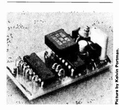
EGGS WITH CHIPS. The transmitter from one of the glass-fibre eggs referred to in the August issue. This one goes in a swan's egg, but Mr Howey is trying to make smaller transmitters using un-encapsulated i.cs.
