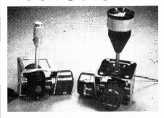
Precise, reliable, long-life Joystick Control Units, in single, dual or triple axis forms. Sprung to centre, or held by adjustable friction locks. Choice of wirewound, cermet or plastic film potentiometers (all standard %" bush types) — or rotary switches.
