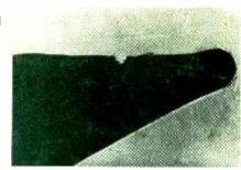
Cracked iron-plated bit, after 40,000 simulated operations using SAVBIT Solder.
