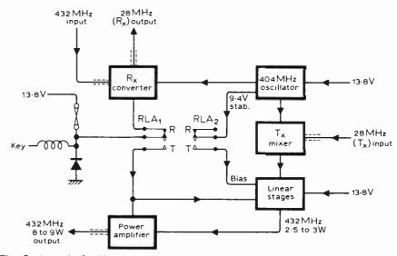
Fig. 2. A typical 432MHz transverter suitable for use with a 28MHz transceiver. This block diagram represents a Modular Electronics design.
