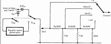
Fig. 7 Practical attenuator. The  $5k940\Omega$  resistors can be formed by a  $6k8//47k\Omega$ , the  $733\Omega$  by a  $6k8//820\Omega$ , and the  $660\Omega$  by a  $22k//680\Omega$ .
