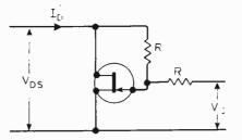
Fig.6. Variable resistor using a f.e.t. The feedback resistor linearises the effective resistance.
