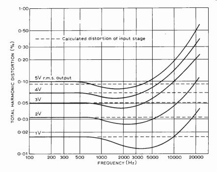
Fig. 10. Open-loop distortion of the preamplifier as a function of frequency and output amplitude.
