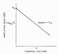
Fig.4. Gain in dB versus control voltage v produces a straight line with the desired characteristic.
