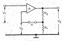
Fig.1. Basic negative feedback amplifier.
