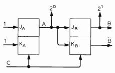
Fig. 3. Two-stage (scale-of-four) counter state diagram and codes (a) and circuit embodiment (b).
