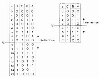
Table 2. Four-bit reflected binary (a) and three-bit (B) reflected binary code.
