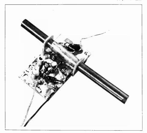
Fig. 2. The complete ferrite aerial unit mounted on a printed circuit board.
