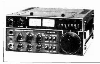
The Icom IC-211E 2m v.h.f. transceiver from Inoue. It uses a patented Icom m.o.s. l.s.i. synthesiser to give v.f.o. tuning on the s.s.b., c.w. and f.m. modes. Other features include repeater facilities and a digital frequency display giving a readout to the nearest 100Hz.
