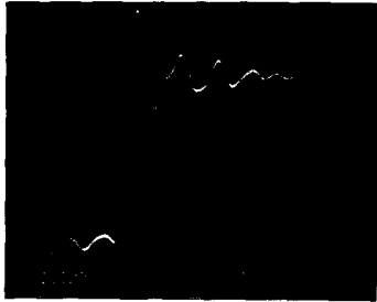
Figure 3-2. The same input signal as shown in figure 3-1, but accessed by a 350 MHz system bandwidth scope (same 6" ground lead).
