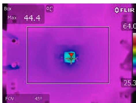
Figure 4. LTM4632 thermal performance. 12V input, 3A. (Figure 2 design)
