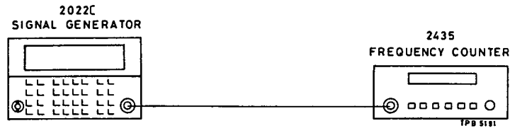
Fig. 5-2 Test gear arrangement to check frequency accuracy
