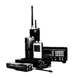
Mobile radios come in many shapes and sizes from hand-held portables to remote-controlled installations. The frequency range may be MF, HF, VHF or UHF; operation may be simplex or duplex; modulation may be AM, FM or  $\Phi$ M.
