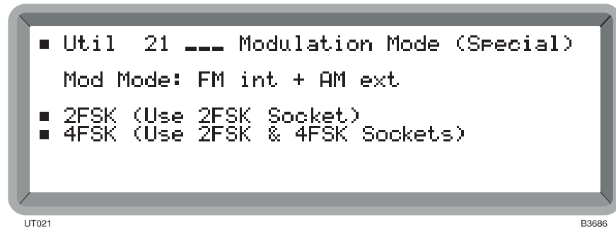
Fig. 4-25 Modulation mode (special) menu
