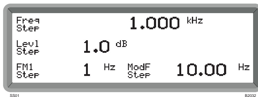
Fig. 4-8 Step setting display showing default settings
