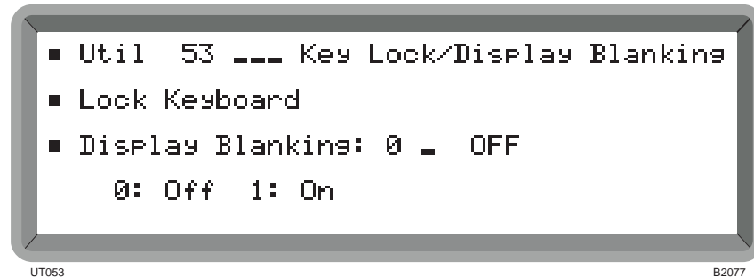
Fig. 4-39 Key lock/display blanking menu
