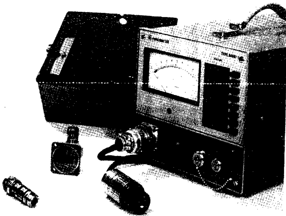
Fig. 1 tft powermeter system showing type 6460/1 with front cover, power head, 20 dB attenuator and coaxial-to-waveguide transformer
