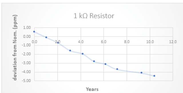
Figure 1 Drift of MI Resistor Over a 10 Year Period
