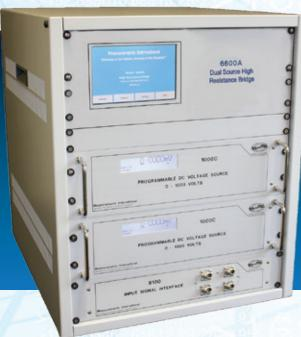
Widest Range Commercially Available  $100k\Omega$  to  $100P\Omega$  Not only does Measurements International offer you the Technology of Choice of Major NMI's for the measurement of World Class Accuracy and Uncertainty levels, but we also offer the complete measurement solution for High Resistance Measurement!
