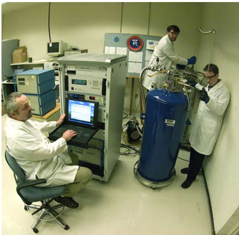
Installation of the Measurements International Quantized Hall Resistance Standard system at the Navy Primary Standards Laboratory, San Diego.
