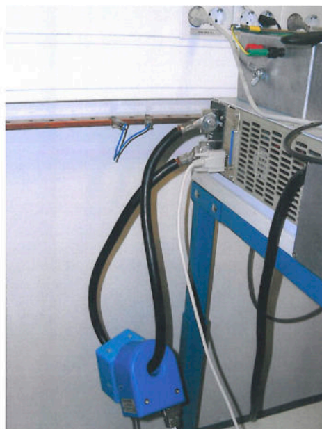
Figure L3: The MIKES ZFCT and the travelling ZFCT connected to the Magna Power (max. 900 A) source. Measurements were done at +90 A, +300 A and +500 A. This setup was not used for calculating the comparison values because the MIKES ZFCT is not yet characterized well enough to be used as a reference on this uncertainty level, but the results still seemed to be within 10 ppm from the actual comparison results
