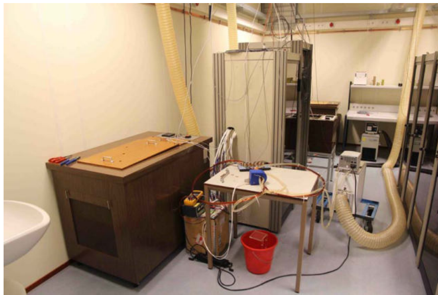
Figure 2. Overview of the VSL measurement setup during the comparison. Measurement rack with low-ohmic resistance bridge (back), water cooling unit (right), oil bath containing R_d resistors (left) and in the front the unit to be measured, the LEM IT-600 S current transformer, with several primary current loops (on the table in the middle). Note the two tubings which removed the heat from the oil bath and water cooling unit respectively, in order to minimise the heat load of the measurement room.
