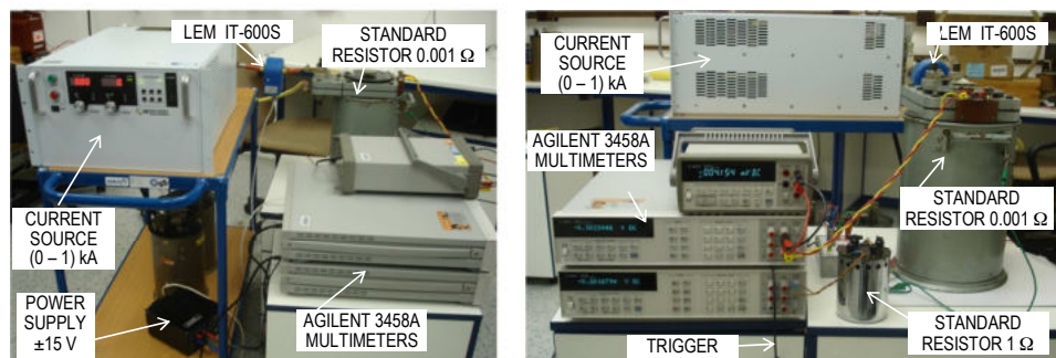
Fig. 2. Workplace for LEM IT – 600S calibration
