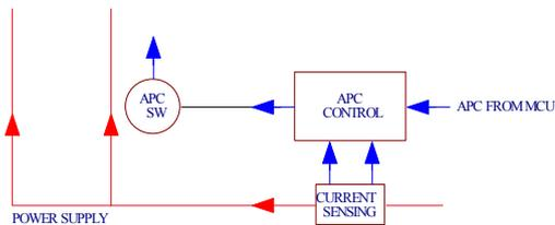
Figure 3.3 APC Circuit Diagram
