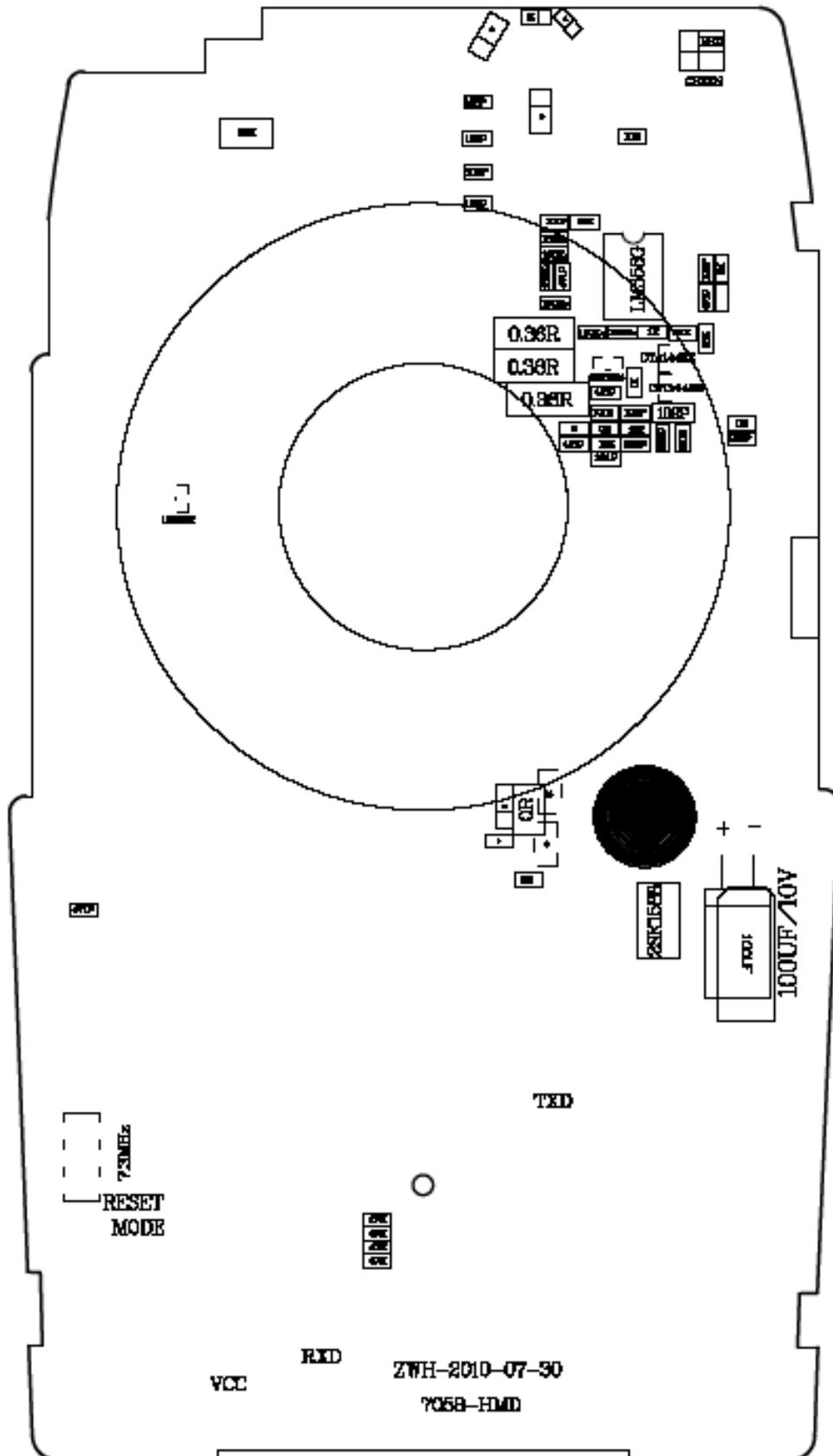
Figure 4 PT260 Top Layer Position Mark Diagram
