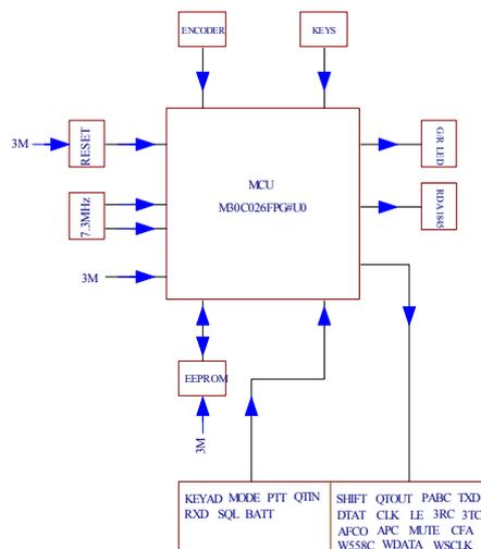
Figure 3.4 MCU Unit Principle Diagram
