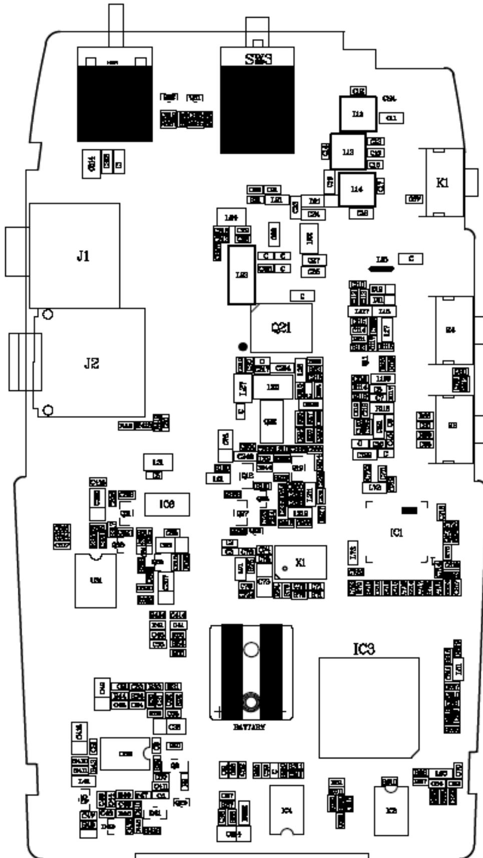
Figure 5 PT260 Bottom Layer Position Mark Diagram
