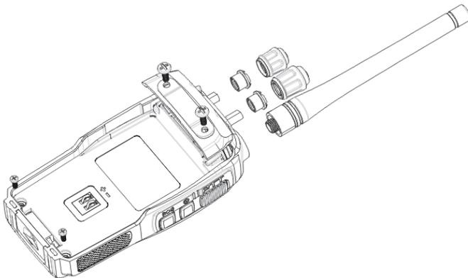
**5.6 Removing the Main Board from the Chassis**
