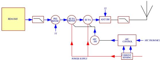
Figure 3.2 Power Amplifier and Antenna Switch Diagram
