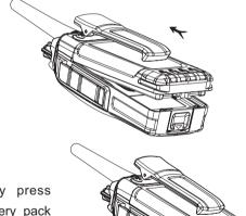
Firmly press the battery pack downwards until the battery latch locks.
