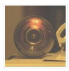
A dekatron was the tube era decade counter "integrated circuit" (IC). It did a full divide-by-10 function, all in one tube. It didn't do it the modern way, by cramming a bunch of components onto a silicon chip, as in a modern semiconductor IC. It did it elegantly using metal structures arranged such that pulsing it, a plasma GLOW would hop, from one electrode, to the next. The added benefit, was that the count position, is visible, thru the top of the tube.
