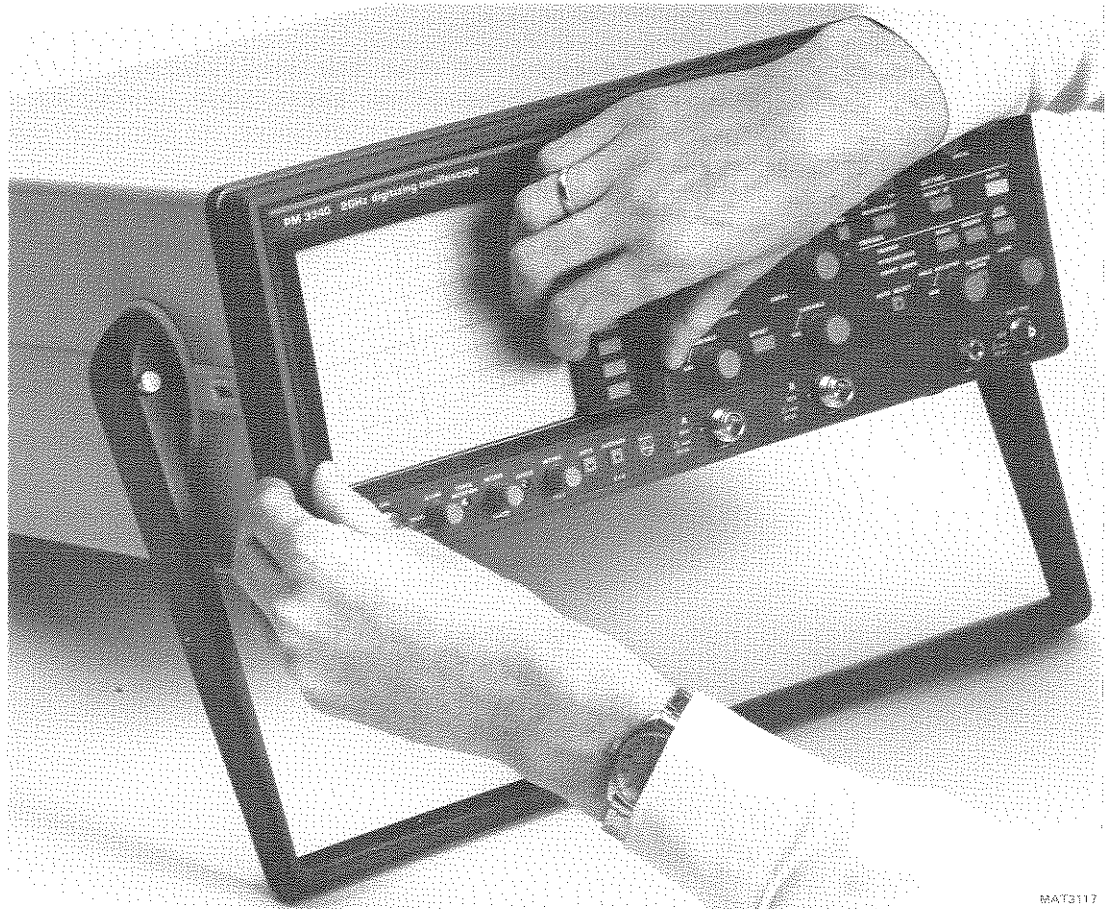
Figure 5.1 Removing the bezel and contrast filter.
