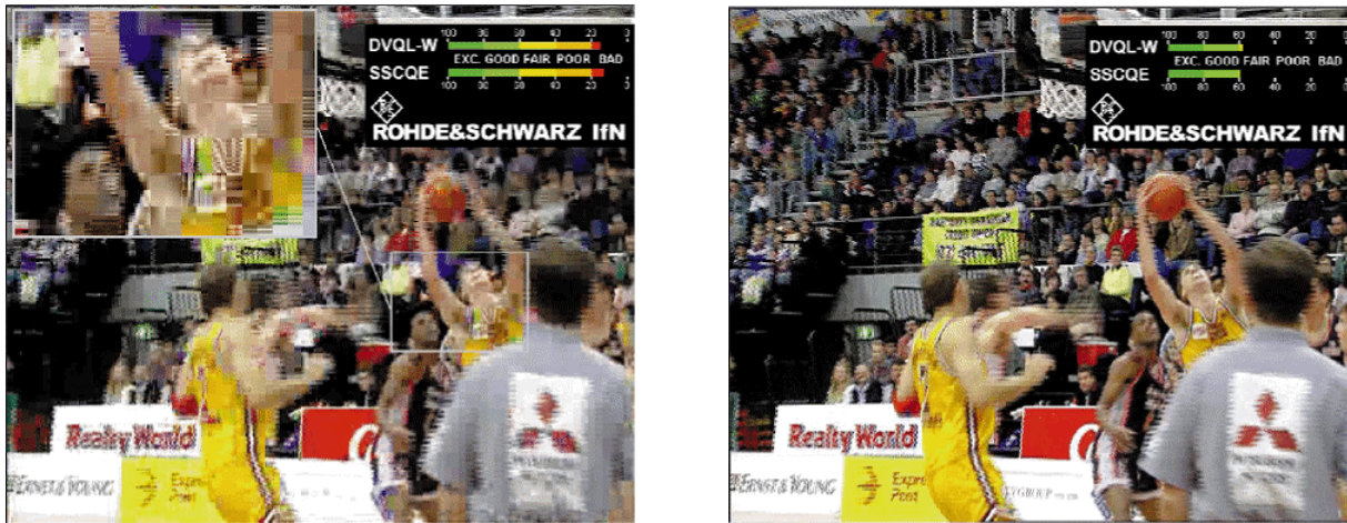
Fig. 1-12 Clearly visible blocking effects on digitally coded TV picture and – by comparison – picture without blocking.
