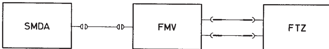
Fig. 3-16 Measurement of modulation distortion with FM and \phi M
