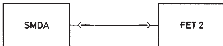
Fig. 3-7 Measurement of modulation-generator frequency
