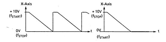
The special function "X-voltage decreasing if fSTART > fSTOP" is switched on using code 41 and off using code 42.
