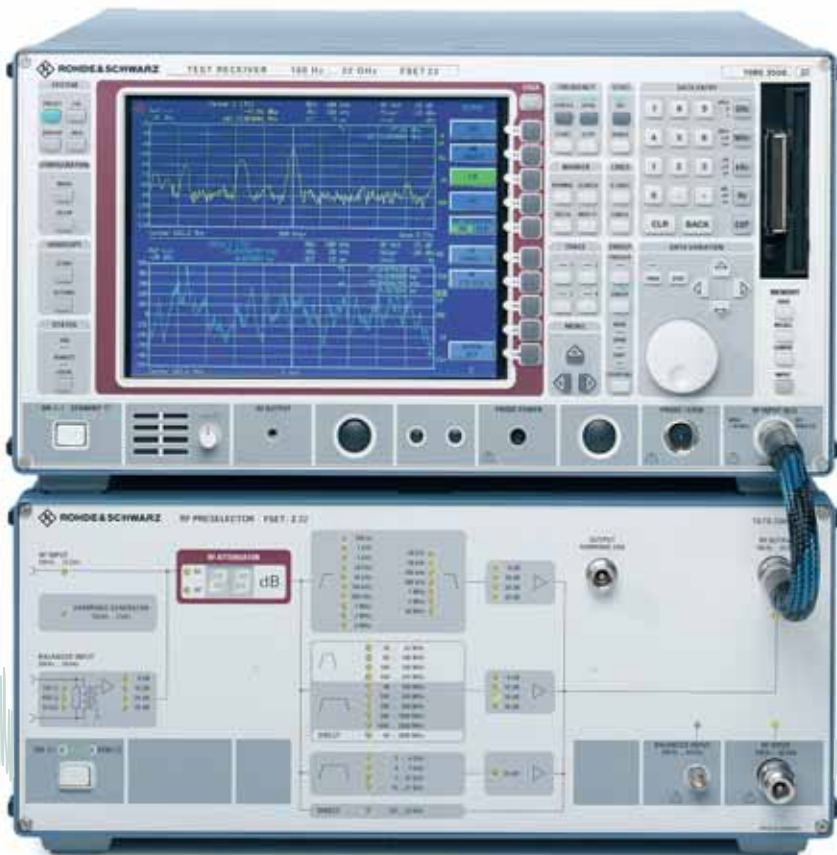
Improved data security and structuring for different user groups by means of a removable hard disk containing measurement results, limit lines, operational system, instrument firmware, etc.
