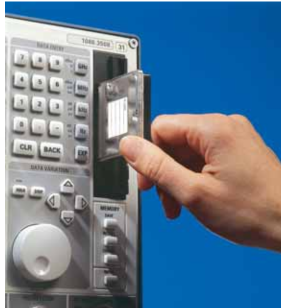
Improved data security and structuring for different user groups by means of a removable hard disk containing measurement results, limit lines, operational system, instrument firmware, etc.
