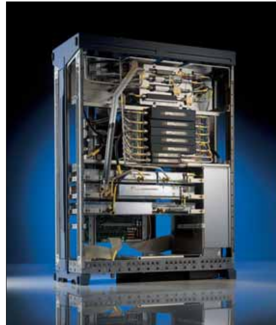
Interior of the RF Preselector R&S FSET-Z22: a glance into the unit shows the complexity of signal filtering. The solid and modular design ensures a long life and great service friendliness.
