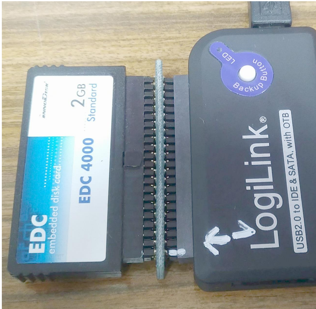
Figure 14: very important: always check for correct orientation! (pin1 )
