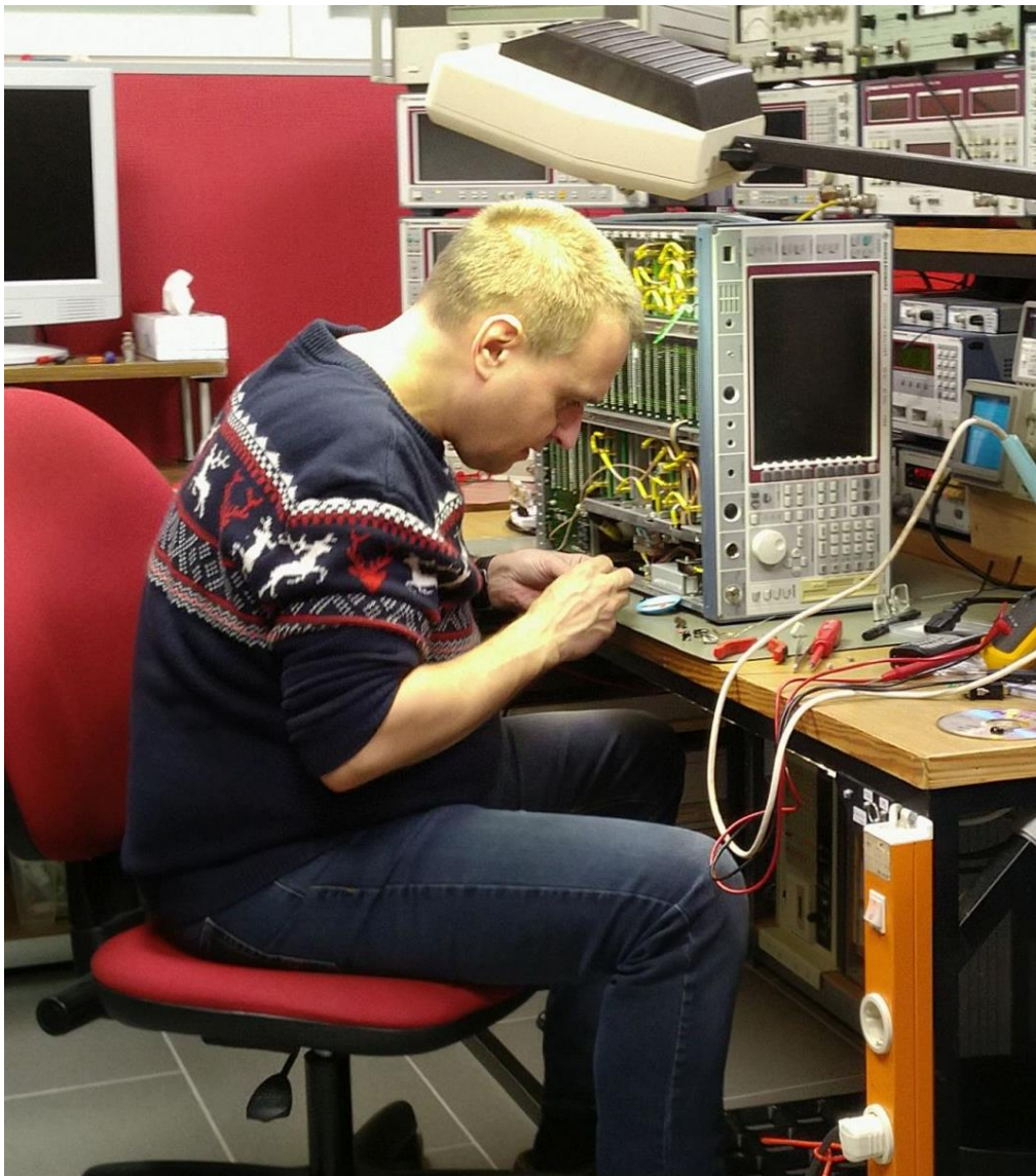
Figure 21: me, Marc DL8ABE, repairing the FSEK power switch (photo: Max Michalzik)
