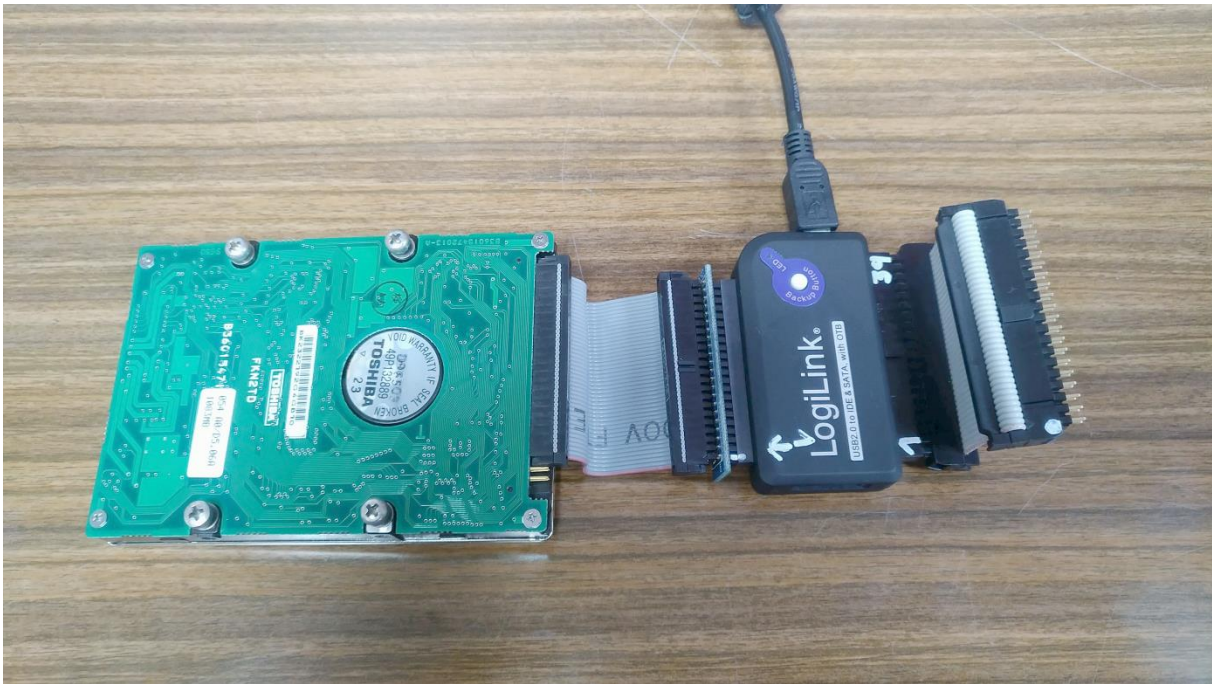
Figure 10: attaching the original FSEK harddisk to the USB interface
