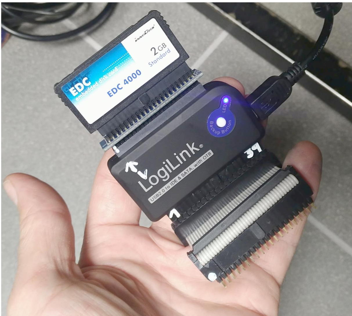
Figure 6: the tools used for the FSEK harddisk replacement – here, shown with a cheap 2GB module
