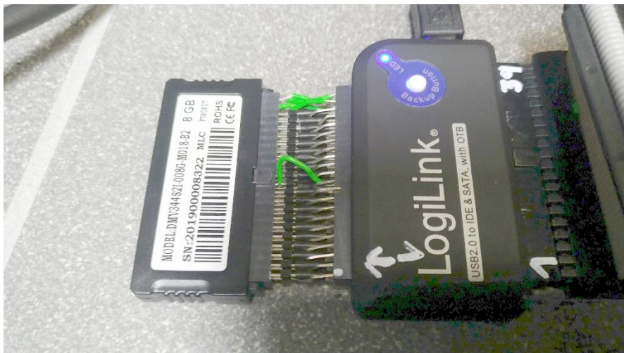
Figure 8: works, but sucks: a selfmade 44pin x-over adaptor
