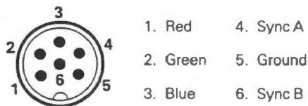
Figure 1 RGB socket, monitor rear view
