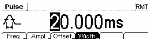
Figure 2-17 Pulse Signal Parameter Setting Interface
