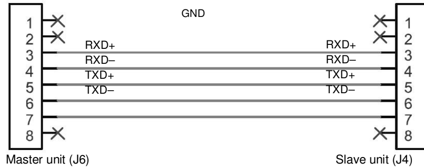
Figure 5-6 RS-485 Communication Cable from Master to Slave Unit
