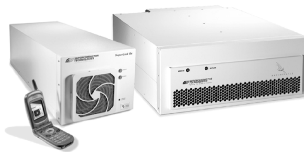
Fig. 8. Size comparison of STI SuperLink Rx (2002) (shown on left) and SuperFilter II (1999) (shown on right) product platforms. Both systems contain control circuitry, a cryocooler, and a dewar with six RF paths (HTS filters plus cryo-LNAs).
