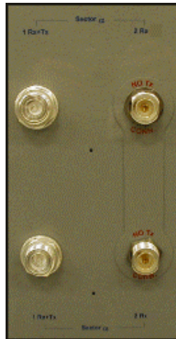
Figure 6. Rx Paths Only Indicated by “No Tx Conn.” Plates
