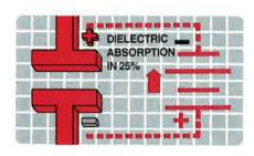
Dielectric Absorption. Dielectric absorption (D/A) is the capacitor's inability to completely discharge. D/A in a capacitor acts as a battery that changes the circuit's bias voltage, and it changes the capacitor's value 'in-circuit'. We found that 25% of the capacitors tested in our study failed because of excessive D/A.
