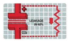
**Leakage.** Leakage develops when the capacitor has an internal parallel resistance that bypasses current through the dielectric. Excessive leakage may cause problems in filtering and high impedance circuits.
