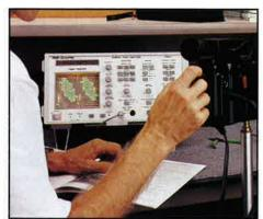
Perform digital vectorscope measurements for easy, error-free color checks. The CVA94 allows you to quickly obtain a vector display and digital measurements of the phase and amplitude of a video camera's chroma output signals. This allows you to confidently tell your customer that the camera's color circuits are working correctly and will produce color that "looks right."
