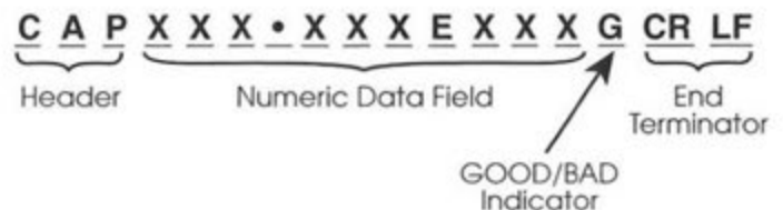
Fig. 19: The data format returned by the LC103 is a string of 17 characters long.
