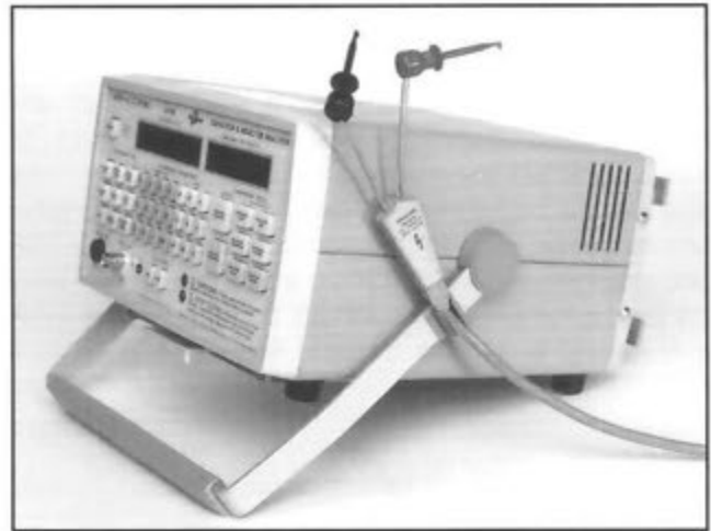
Fig. 9: The test lead mounting clip holds the test leads out of the way, yet ready for use at anytime.
