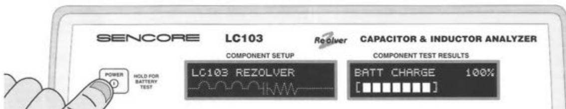
Fig. 7: Press and hold the Power button to read the remaining battery charge.
