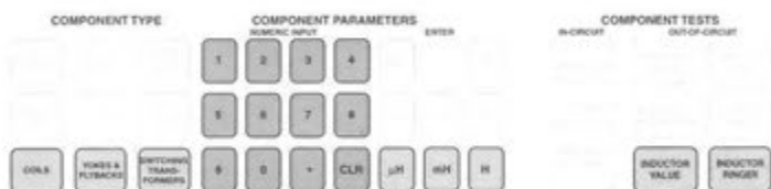
Fig. 15: Controls used for out-of-circuit inductor testing.
