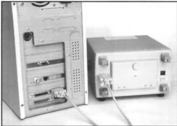
Fig. 17: Connecting the LC103 to a computer for automated control.
