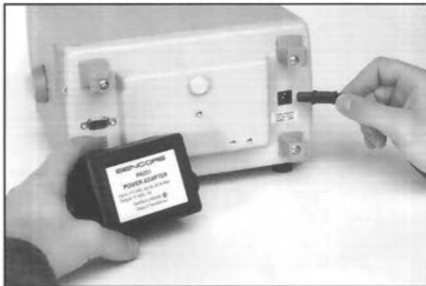
Fig. 5: Connect the PA251 to the 12 VDC input for AC bench operation and to recharge the optional battery.
