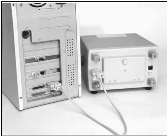
Fig. 17: Connecting the LC103 to a computer for automated control.
