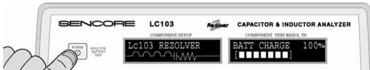
Fig. : Press and hold the Power button to read the remaining battery charge.
