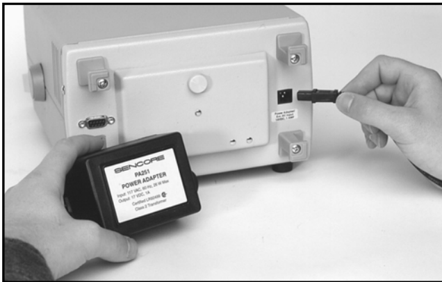
Fig. 5: Connect the PA251 to the 12 VDC input for AC bench operation and to recharge the optional battery.
