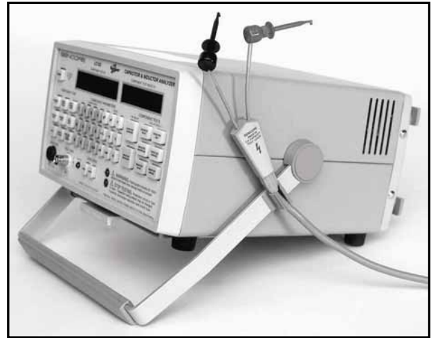
Fig. 9: The test lead mounting clip holds the test leads out of the way, yet ready for use at anytime.
