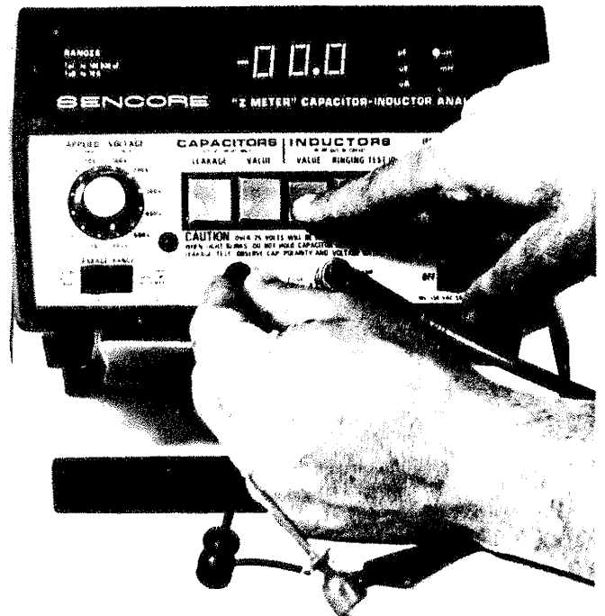
Fig. 18 — The inductance of the test leads can be balanced out for accurate readings of small value inductors.
