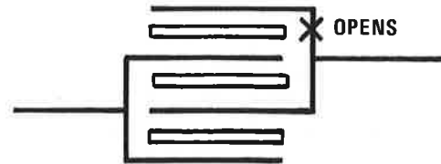
Fig. 39— A break in one of the foil connections to the lead of a multi-layer foil capacitor can reduce the capacity value.
