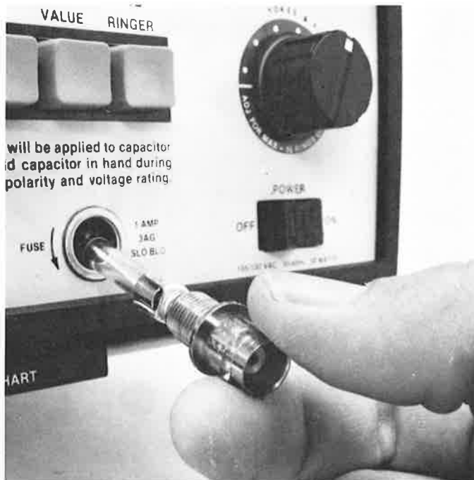
Fig. 5— A 1 amp 3AG slo-blo fuse protects the LC75 input. The fuse is located behind the test lead input jack.
