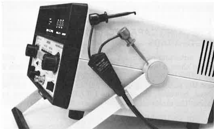
Fig. 6— The test lead mounting clip holds the test leads out of the way, but ready for use.
