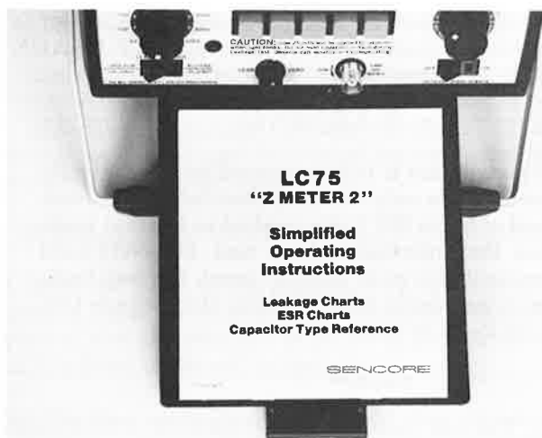
Fig. 12— Consult the leakage charts on the pull chart under the LC75 or the leakage charts in this manual for the maximum allowable leakage of aluminum and tantalum electrolytics.
