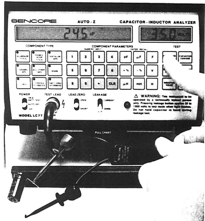
Fig. 15 — To measure capacitance, connect the capacitor to the test leads and push the CAPACITOR VALUE button. The amount of capacity appears in the LCD display.
