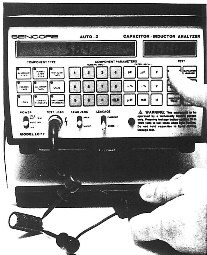
Fig. 20 — The LC77 provides an automatic good/bad indication of each capacitor parameter.
