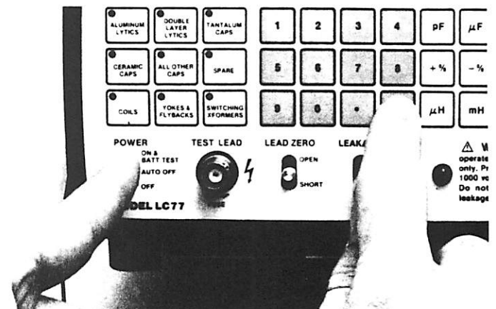
Fig. 67 — Push the "CLR" button while holding the power switch to "ON & BATT TEST" to check LCD display.
