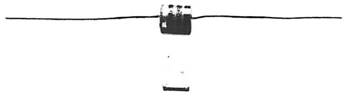
Fig. 48 — Ceramic capacitors may also include an axial lead and chip-type package. Axial lead ceramics often look like other axial lead components.
