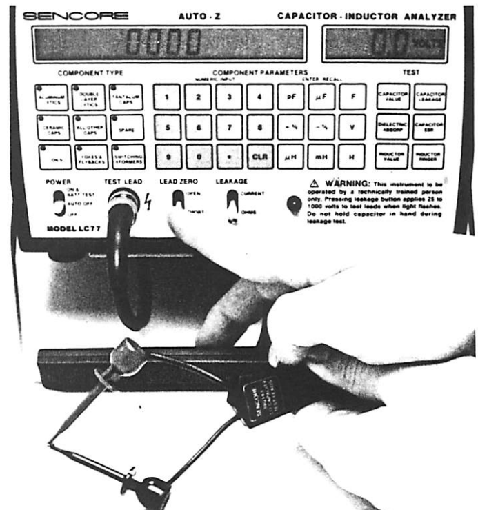
Fig. 22 — Connect the test leads together and push the LEAD ZERO button to “Short” to balance out the test lead impedance when checking small value inductors.
