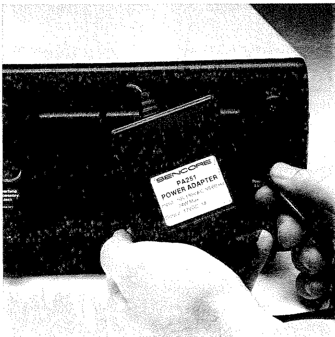
Fig. 6 — Connect the PA251 to the 12 V DC input for AC bench operation and to recharge the optional battery.
