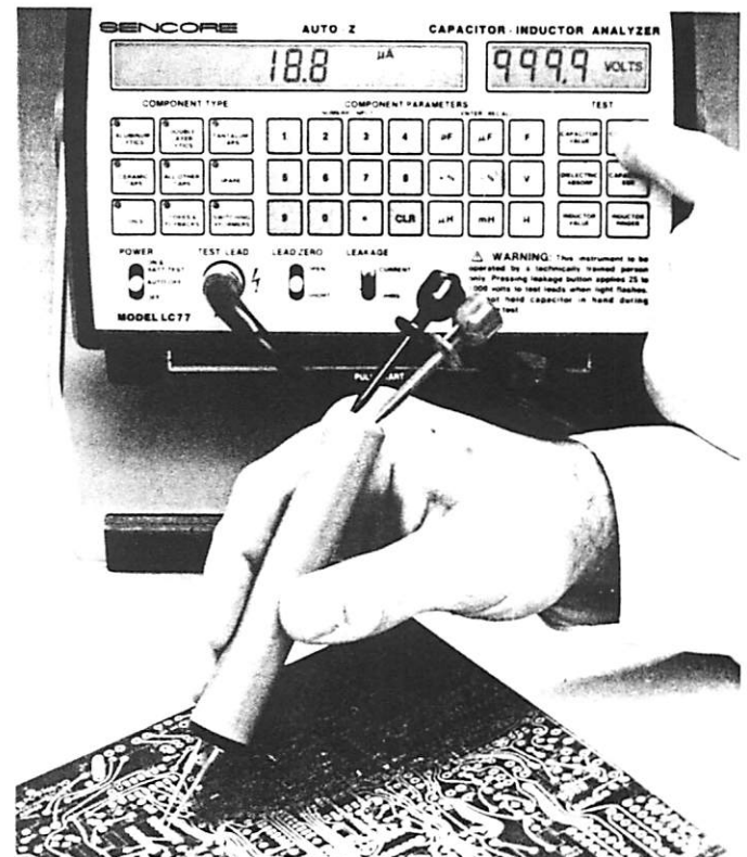
Fig. 65 — Small leakage paths can be detected with the LC77 Hi Pot test.
