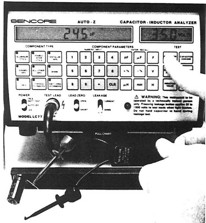
Fig. 15 — To measure capacitance, connect the capacitor to the test leads and push the CAPACITOR VALUE button. The amount of capacity appears in the LCD display.
