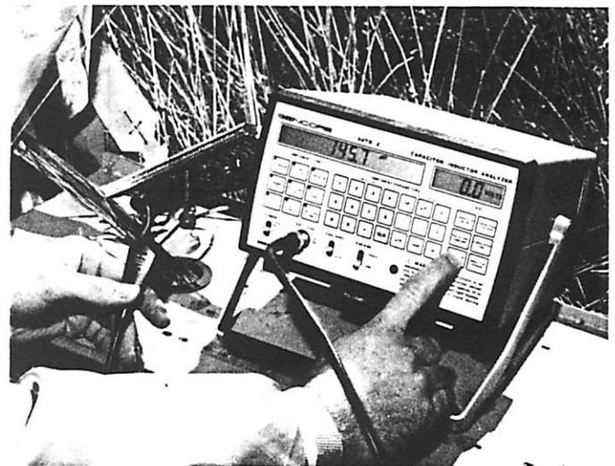
Fig. 64 — Use the LC77 to measure the distance to breaks or shorts in buried cable.
