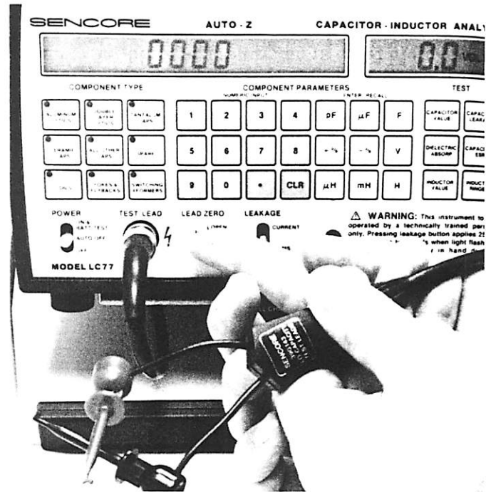
Fig. 11 — The impedance of the test leads is balanced out with the LEAD ZERO button.
