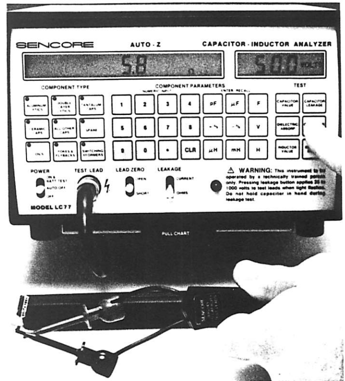
Fig. 18 — Depress the ESR button and read the amount of ESR in the LCD display.
