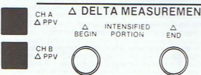
Fig. 51 — The amplitude of any part of the channel A or B waveform is measured by pressing the correct button and adjusting the BEGIN and END controls until the Delta Bar covers the area to be measured.
