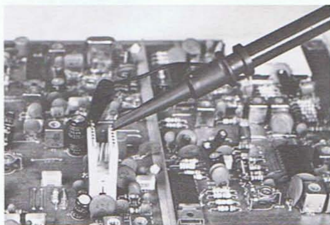
Fig. 18 — IC test clips provide secure connections to IC pins with little chance of shorting adjacent connections.
