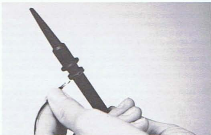
Fig. 20 — Make sure the ground clip is centered in the strain relief hole before trying to remove the clip.
