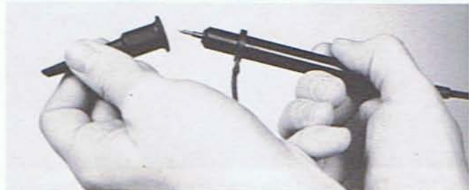
Fig. 17 — Unscrew the probe tip to expose a sharpened steel probing tip.
