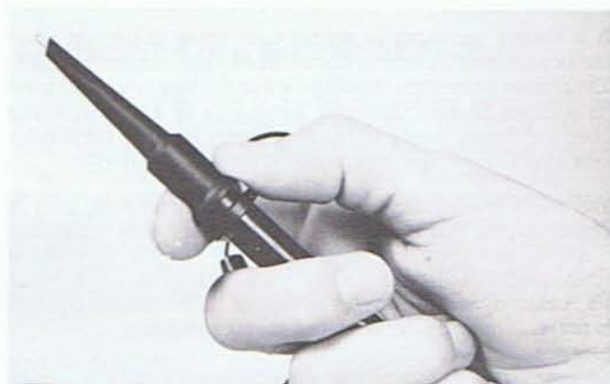
Fig. 16 — Pulling back on the collar exposes the metal hook that is connected to the circuit.
