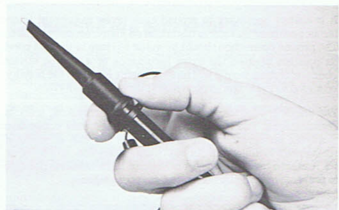
Fig. 16 — Pulling back on the collar exposes the metal hook that is connected to the circuit.
