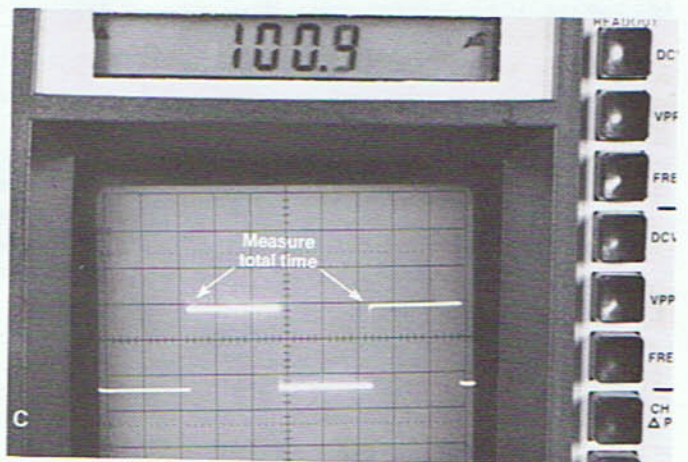
Fig. 55 — Duty cycle is measured by comparing the on-time to the total time of a waveform. Note that only one Delta position needs to be changed to expand the Delta Bar.
