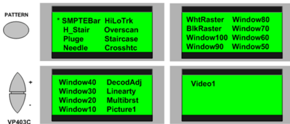
Figure 4. Push the “-” scroll down button on the VP403C to select the last menu. Press the pushbutton beside the display indicating “Video 1” selection.
