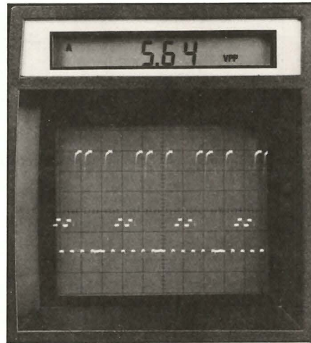
Fig. 7: The data at each pin will appear to be out of sync because it is constantly changing. Concentrate on the fact that each pin is toggling, and not stuck at logic high or low.
