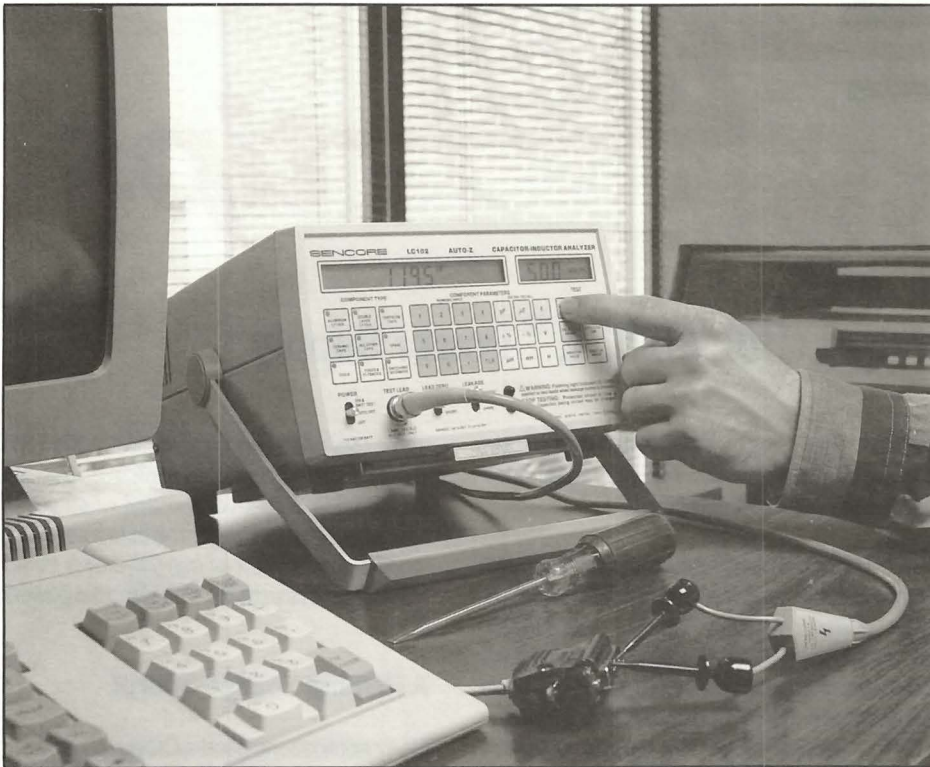
Fig. 2: When tracing a wire in a cable, connect the LC102 at one end, while you look for the DC voltage with a meter at the other end.
