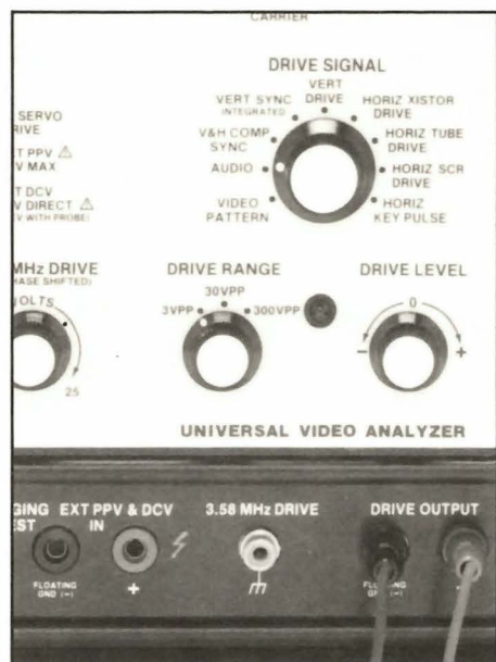
Fig. 9: You don't need to disconnect components when using the Drive Signals, because the VA62A swamps out the signal in the circuit.
