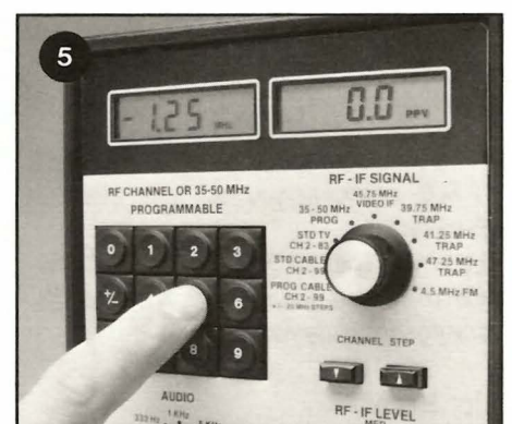
Fig. 4: The Programmable Cable function lets you program each cable channel with an offset. 1. The channel number shows before entering the program mode, 2. The display shows the current frequency program (zero indicates no program), 3-5. Entering the desired numbers program in a new frequency offset.
