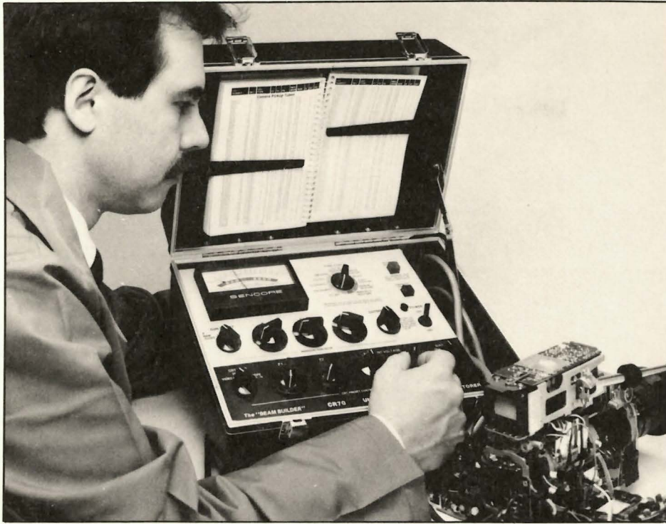
Fig. 4: The Universal Adapter and the CR70 let you test mounted camera tubes.
