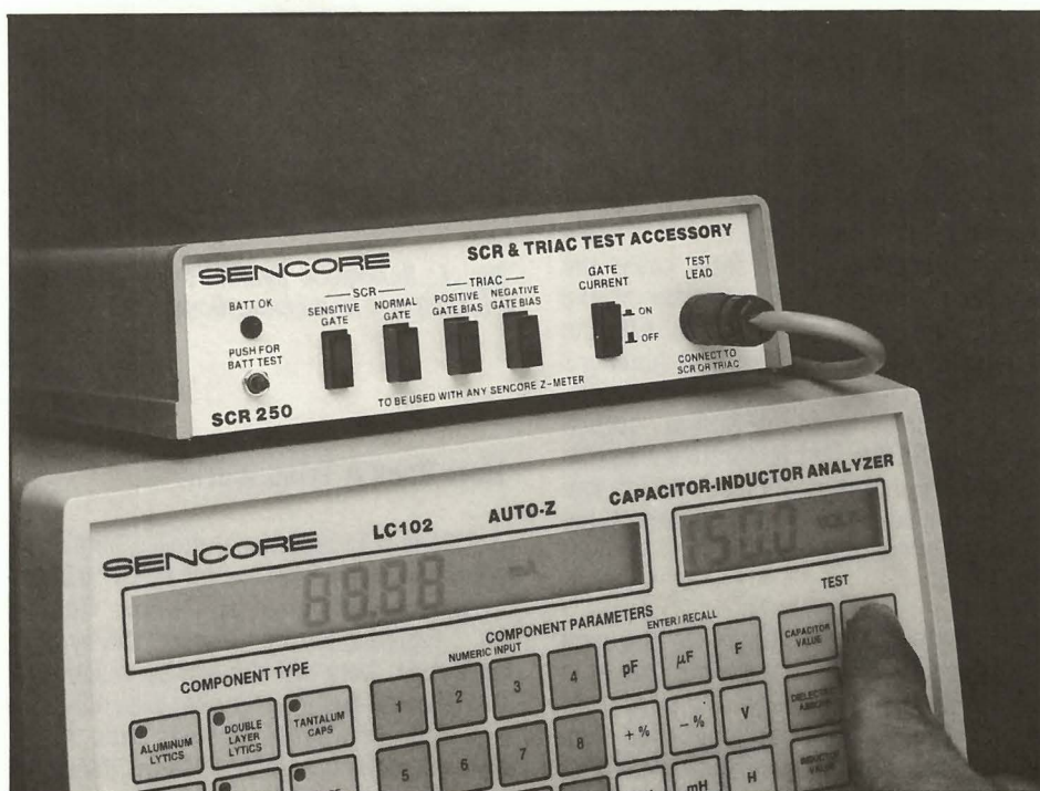
Fig. 3: Testing the SCR at the working voltage may show leakage when it wouldn't at a lower voltage.
