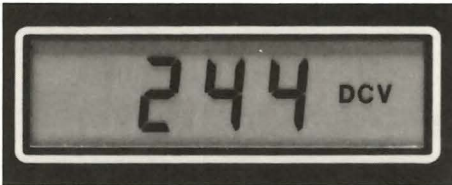
Figure 1: Simply multiply the VA62A's digital meter reading by 100 to obtain the value of the voltage being measured. For the example shown, the reading of 244 volts represents a circuit voltage of 24,400 volts.
