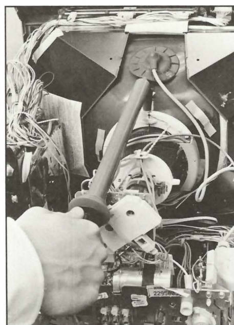
Figure 3: The HP200 should be connected to the circuit so that you do not have to hold on to it, but if this is not possible, only hold it by the black handle as shown.
