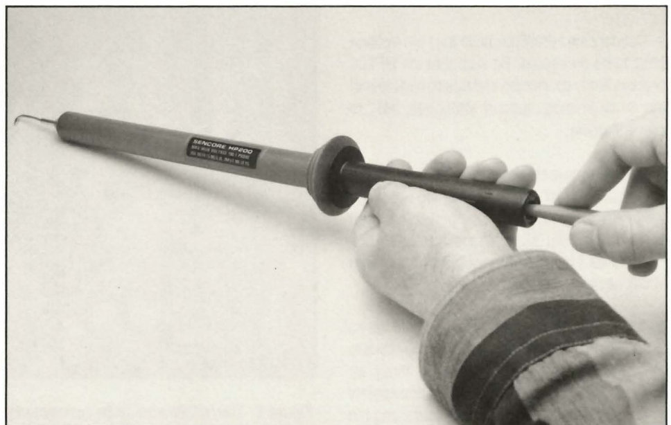
Figure 2: The HP200 fits over the end of the regular test probe and increases the measuring capabilities to 50,000 volts.
