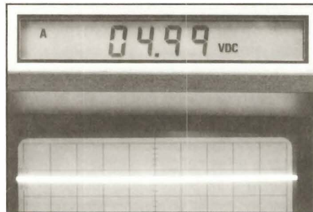
Fig. 3: Use the SC61's DIGITAL READOUT DCV function to measure the output of single logic change sensors.
