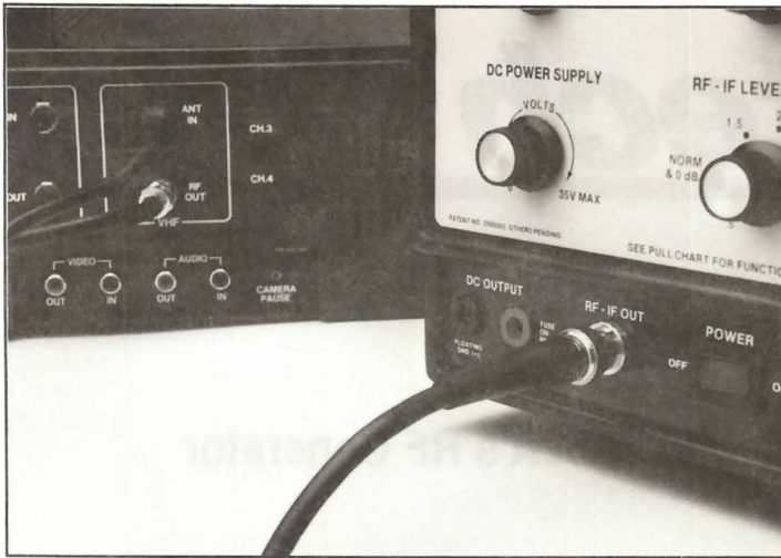
Fig. 2: Connect the RF-IF OUT of the VA62A to the antenna in on the VCR, and set the tuner to the proper sideband.
