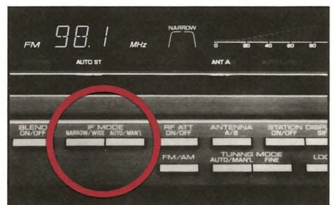
Fig. 8: User-selectable IF bandwidths let the listener narrow the response for weak stations, or widen the bandwidth for highest fidelity on strong RF signals.
