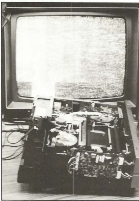
Fig. 4: A failure in just one head channel produces a picture that has noise throughout the entire screen.
